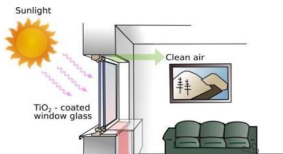
Figure 3. Windows with nanostructured coatings can cure 'sick' buildings.
